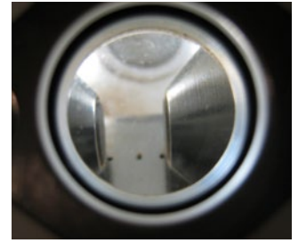
Nano-particle coated sensor optics and the flow cell looked visually clean.
